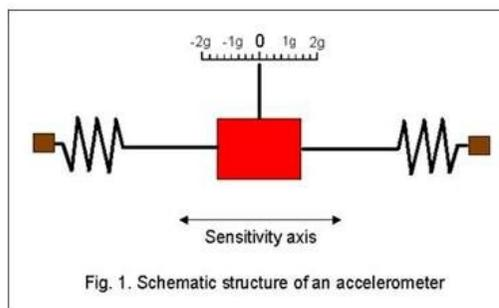
In Newton's day, accelerometers were built using a test mass (shown in red) held at rest with springs and having a scale showing the acceleration along the sensitivity axis. Note that the unit (**g**) is equal to the acceleration subject to all bodies at the surface of the earth due to gravity, and is equal to about 9.8 meters per second per second. The same gravity is the acceleration that translates our body mass to a weight we can measure when we stand on a scale.
