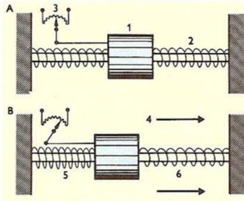
When the system is moving at a constant speed it gives the same result as a stationary system: the mass remains in the middle and at equilibrium with the springs ie *no relative acceleration*.
